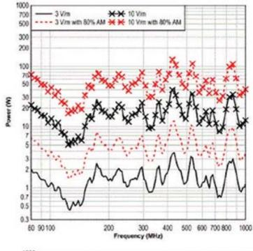
3143B BiConiLog Antenna Typical Average Power Required in Vertical Polarization at 3 m
